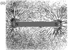
(iii)The direction of a magnetic field at a point is determined by placing a small compass needle. The N - pole of compass indicates the direction of magnetic field at that point.
