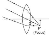
Object at infinity, rays parallel to themselves but not parallel to principal axis. Image is formed at F', the focus on the other side of lens. Object beyond 2F. When the object is beyond 2F, a real, inverted, diminished image is formed between F and 2F.
