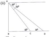
The distance between two positions of ship after 6 seconds CD = BD - BC  $\Rightarrow CD = 40\sqrt{3} - 40 = 40(\sqrt{3} - 1)$  $\Rightarrow CD = 29.28 \text{ m}$
